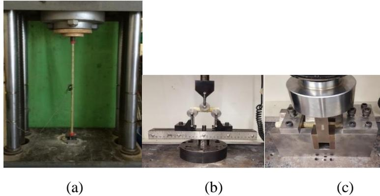
Figure 3. Test setups for measuring (a) Tensile properties (b) Interlaminar shear strength (c) Transverse shear strength
