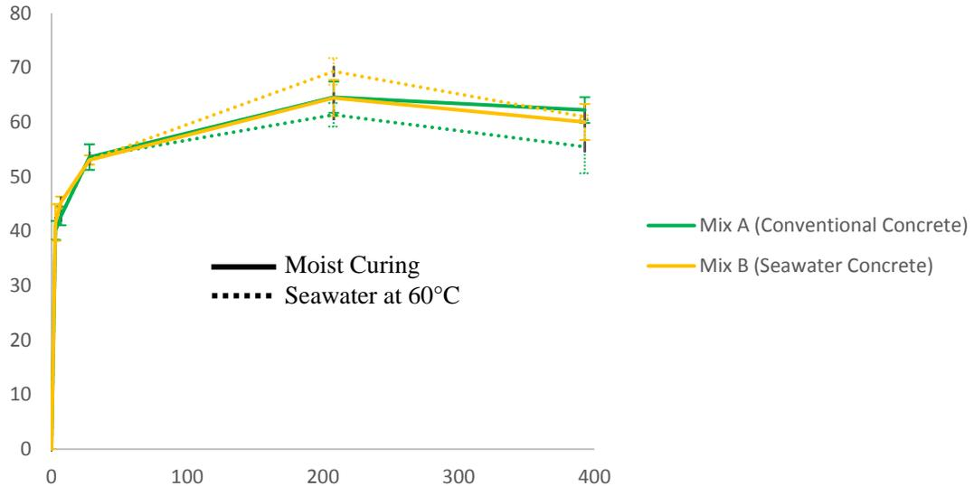
Figure 4. Compressive strength after one-year exposure to control and accelerated conditioning
