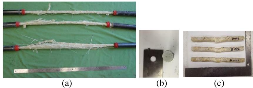
Figure 5. Typical failure mode of the extracted GFRP bars subjected to (a) Tensile test (b) Interlaminar shear test (c) Transverse shear test
