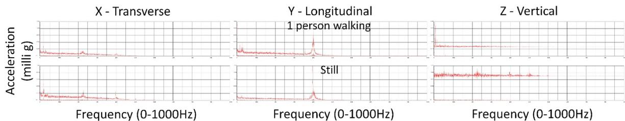
Figure 3 Frequency pattern 0-1000Hz with and without pedestrian traffic
