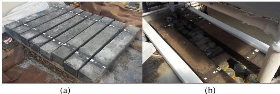
Figure 2: (a) Test beams (b) Seawater chambers for accelerated conditioning
