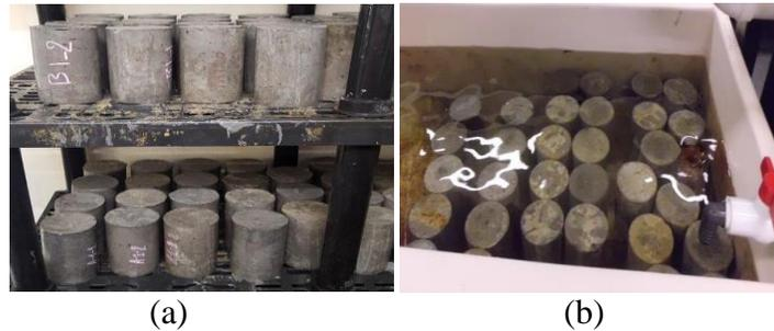
Figure 1: Exposure conditions (a) Control environment: moist curing room (b) Accelerated condition: seawater at 60 °C
