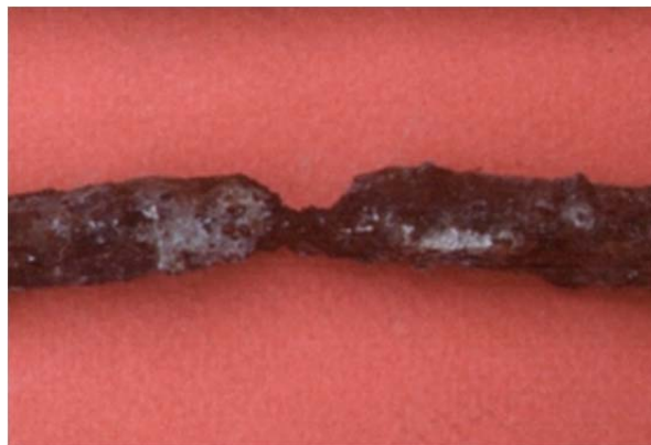
Figure 2 – Example of pitting corrosion of steel bars.
