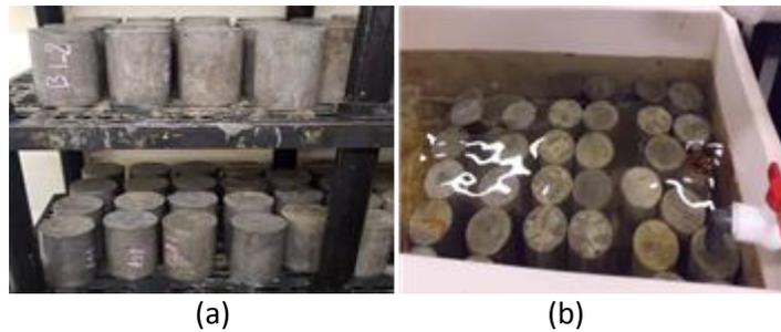
Figure 1 Exposure conditions (a) Control environment - moist curing room (b) Accelerated conditioning environment - seawater at 60 °C
